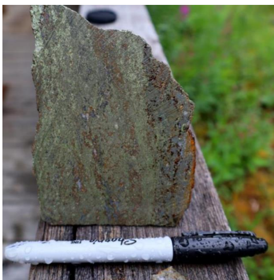
Figure 5: Photo of the massive sulphide float (dominantly chalcopyrite with minor galena)
