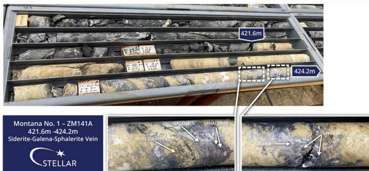
Montana No. 1 Drillhole ZM141A, Fissure Vein from 421.6m to 424.2m with visual sulphide galena and sphalerite mineralisation containing, lead, zinc, silver, copper and tin 3
