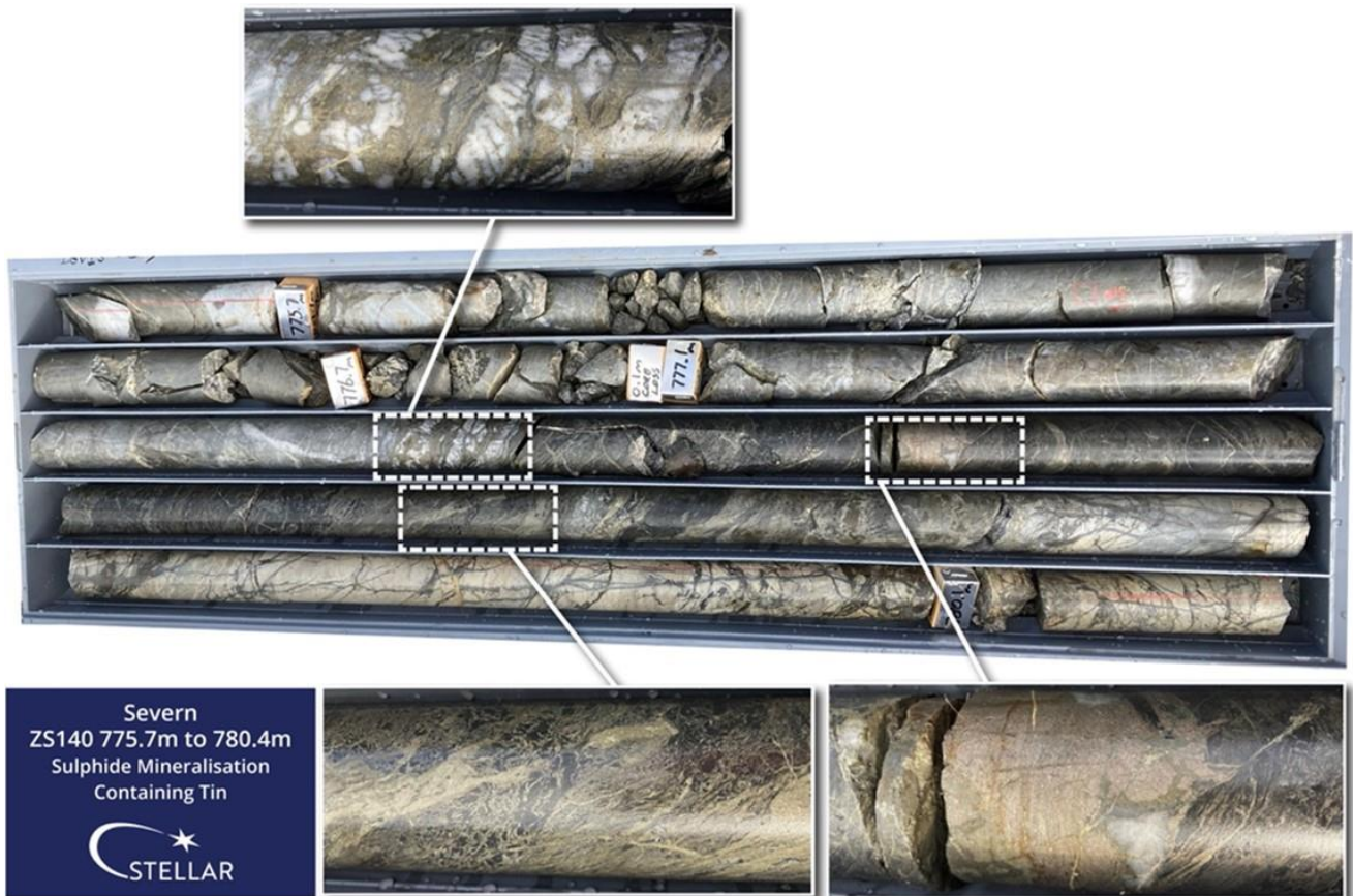
Severn Drillhole ZS140, Typical example (775.7m – 780.4m) of sulphide mineralisation containing tin 3
