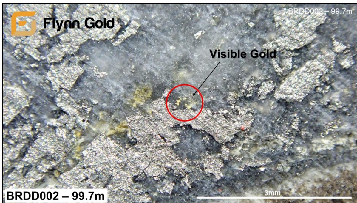
Figure 4: Visible gold associated with arsenopyrite from 99.7m in drillhole BRDD002 (0.5m @ 12.2 g/t Au).
