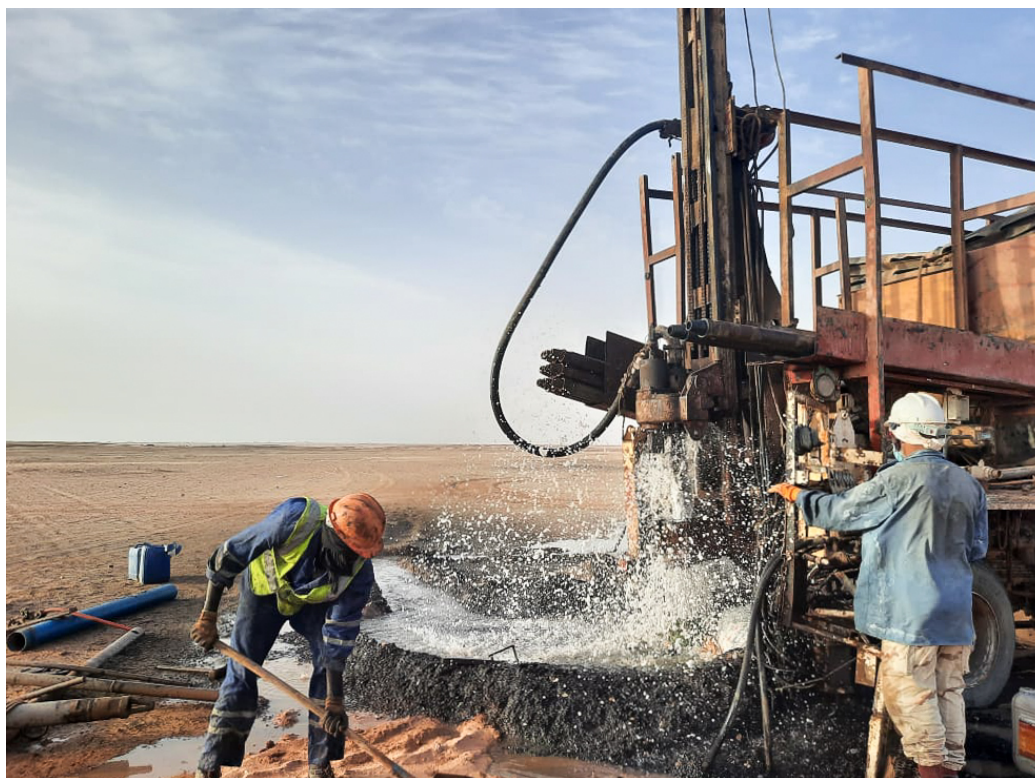
Image 1 – Water drilling underway at Tiris
