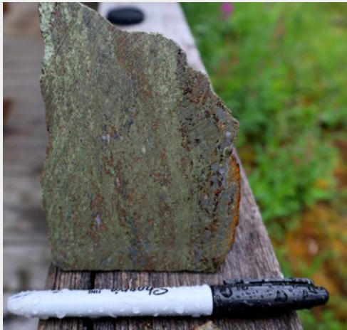
Photo of the massive sulphide float (dominantly chalcopyrite with minor galena) from the Kiwi prospect 2 .
