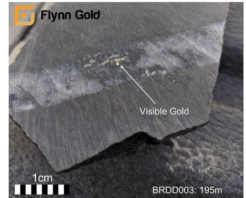
Visible gold associated with arsenopyrite from 195m (0.5m @ 56.3 g/t Au) BRDD003
