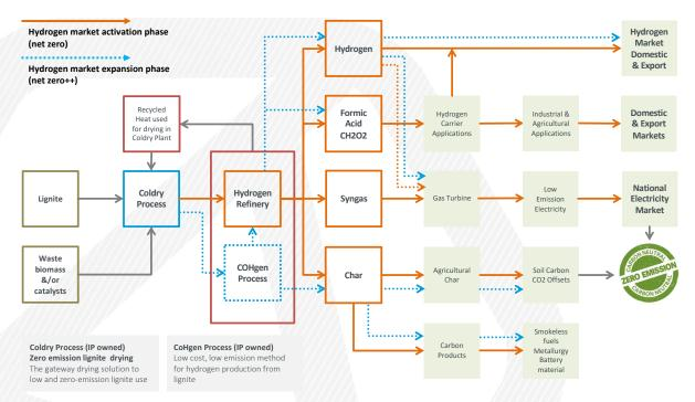
**Diagram (above):** the project involves two phases; Phase 1 entails hydrogen industry activation via an integrated utilisation pathway at scale enabling the manufacture of hydrogen and formic acid. Building upon this foundation, Phase 2 entails hydrogen industry expansion, developing and deploying our proprietary COHgen technology, which represents a significant advancement on conventional hydrogen production methods, featuring 70% lower CO<sub>2</sub> emissions.
