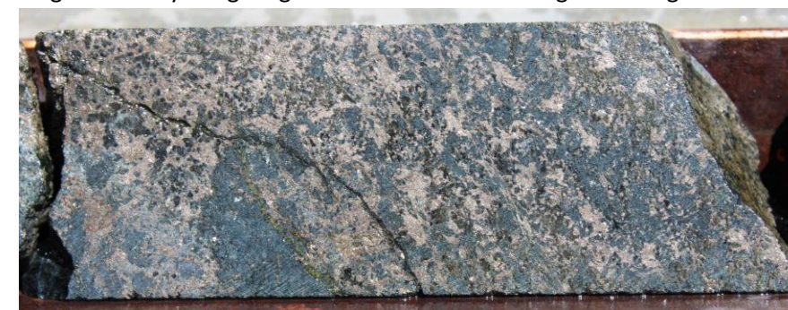
Above: CNDD001A at 635.9m down-hole showing matrix-textured sulphide zone
