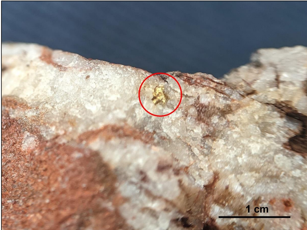
Figure 2. Photograph of visible gold in ferruginous quartz veined sandstone (sample 22566), Trafalgar prospect. Preliminary assay grade of 61.0 g/t Au.
