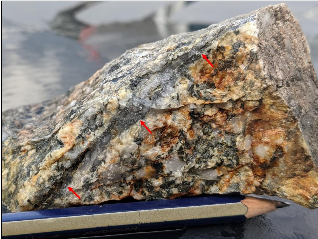
Figure 4. Photograph of quartz-arsenopyrite fracture-veining (red arrows) in altered granodiorite (sample 22565), Trafalgar prospect. Preliminary assay grade of 10.9 g/t Au.
