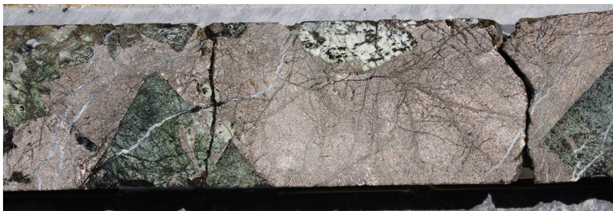
Figure 1: Semi massive sulphide intersected in CNDD001A at 662.1m (part of 0.6m interval containing 0.96% Ni)
