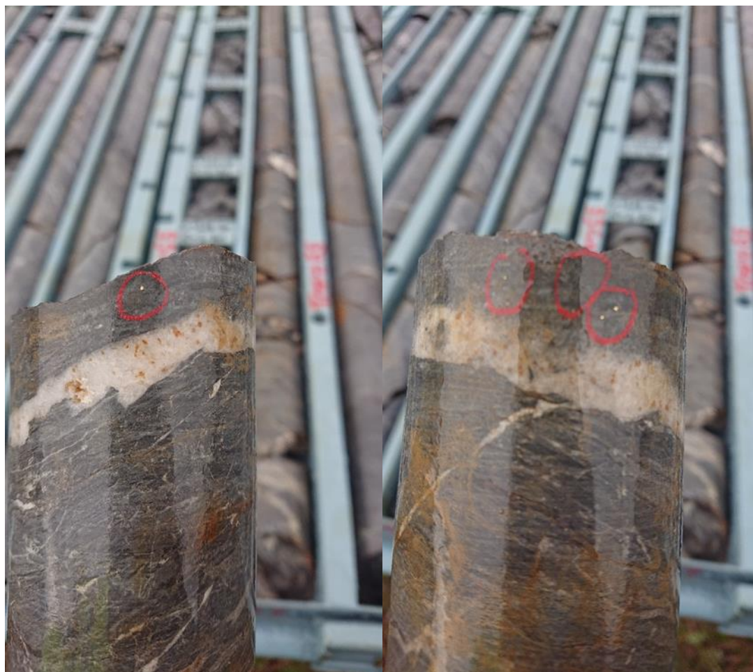
Figure 2: Coarse grained visible gold in heal shear (SUN057)
