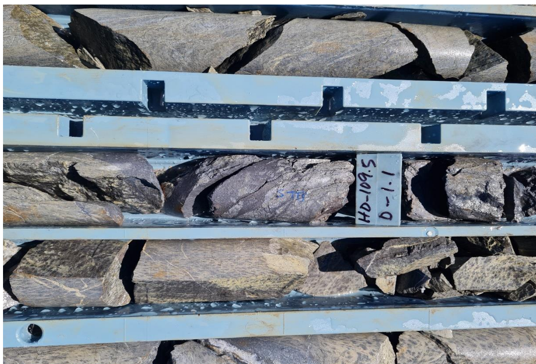
Figure 5: Massive stibnite in core of ELG160
