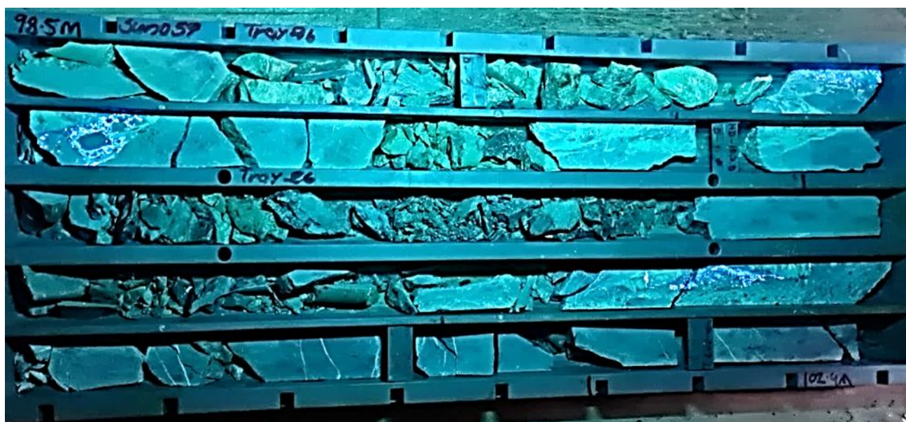
Figure 3: Scheelite (Tungsten) showing fluorescence under UV light in core of SUN057
