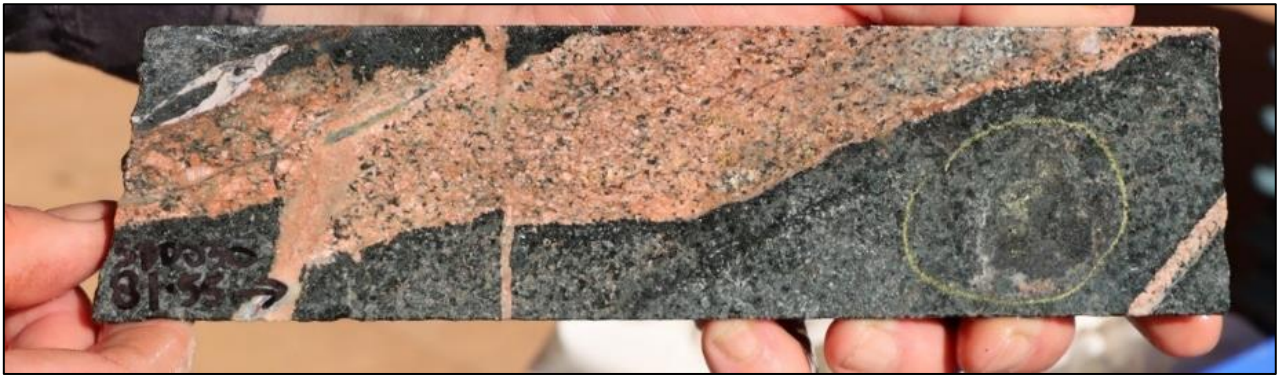
Sunrise East drill core from SDD030 – highlighting pyrite and minor disseminated chalcopyrite associated with monzonite dyke.
