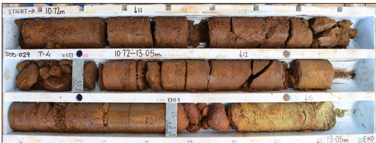
Cobalt-rich laterite core from Sunrise East SDD029.
