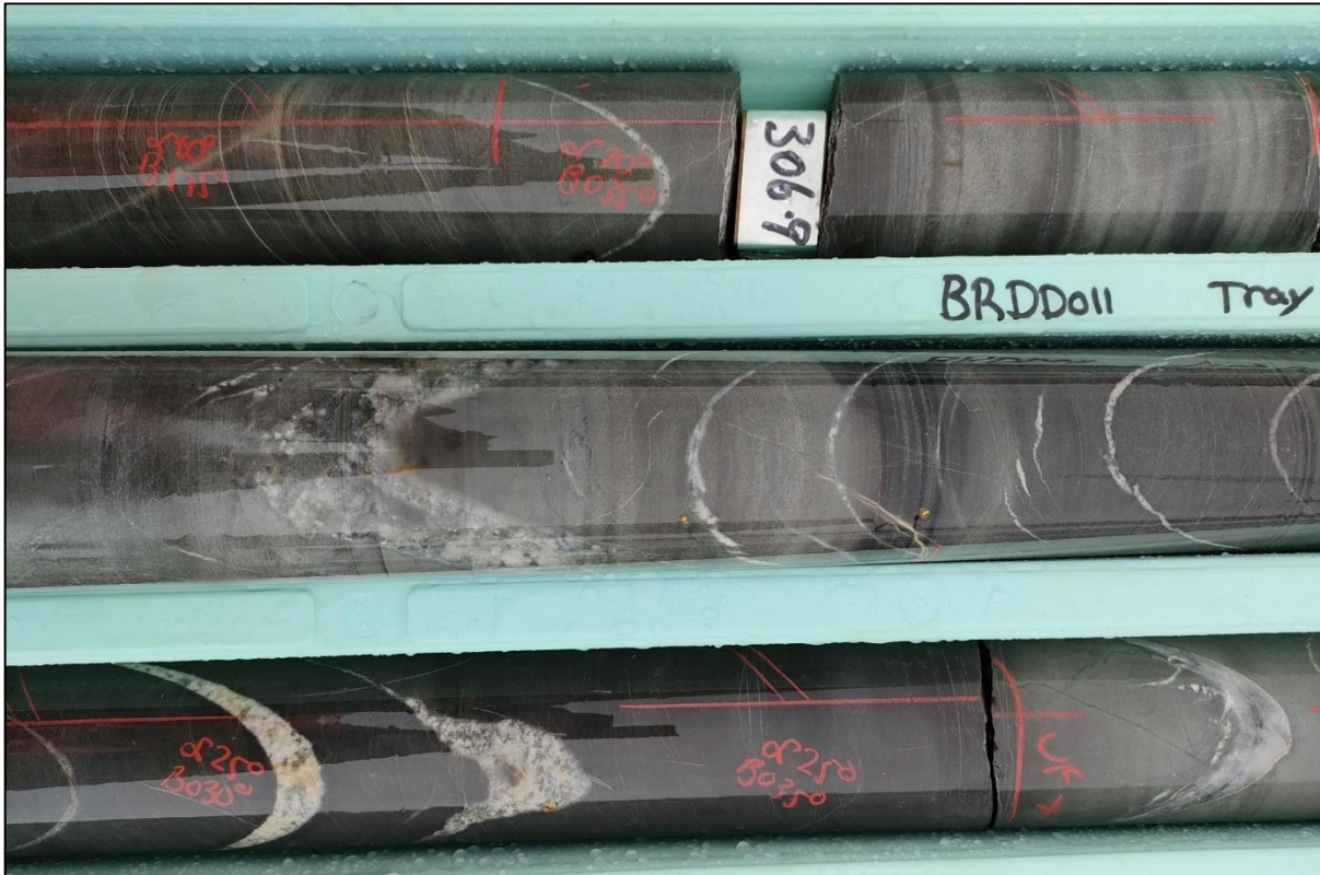
Figure 3. Example of arsenopyrite mineralised veins in BRDD011 – intercepted in the predicted down-plunge extension zone.
