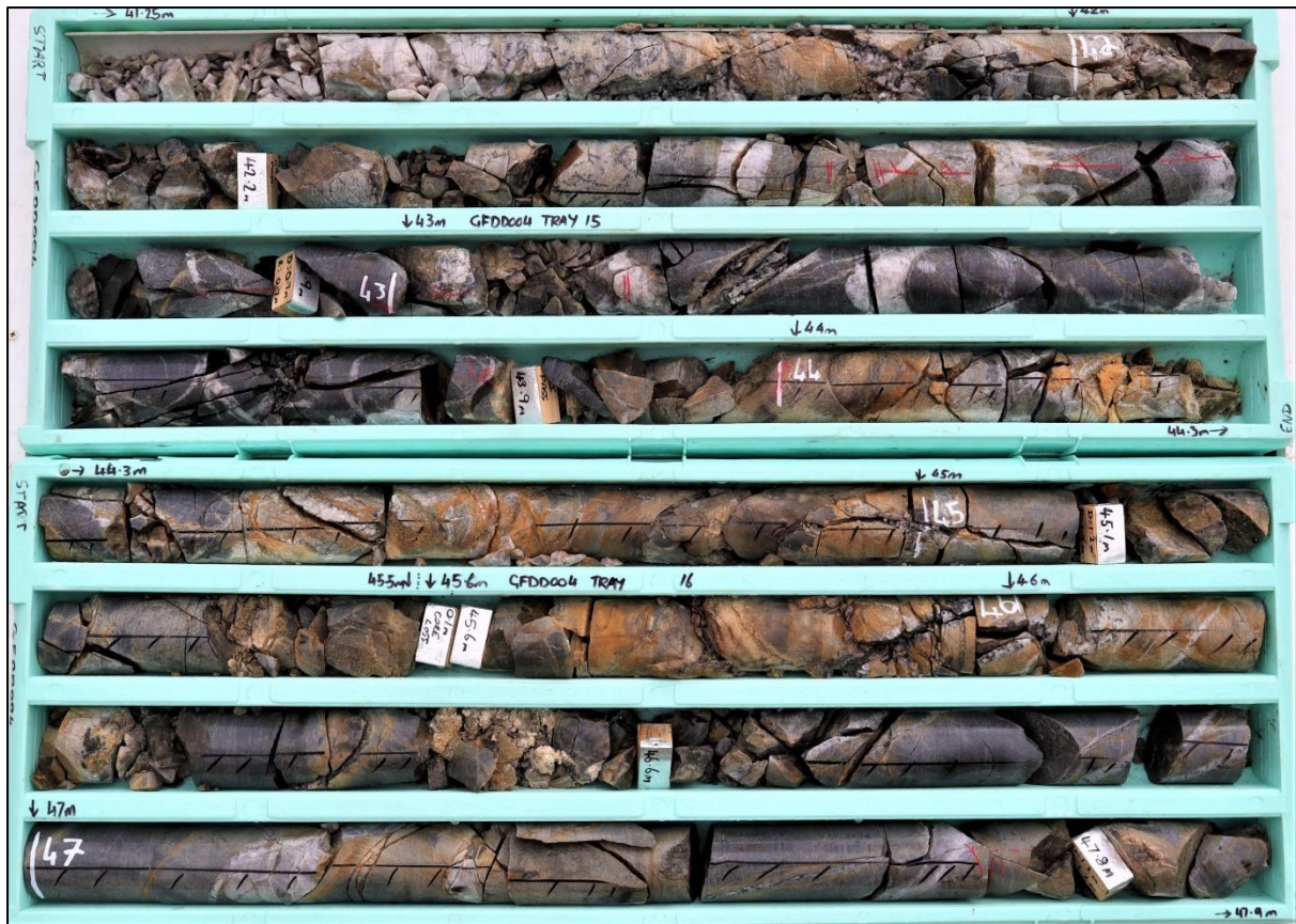
Figure 10: Photograph of drill core from GFDD004, Grand Flaneur prospect, showing quartz-sulphide veining in strongly ferrous carbonate altered silicified channel sand host unit. Interval shown includes 1.4m @ 9.66 g/t Au from 45.6m .
