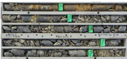
Composite 7 – 37.8 to 43.5m Coarse Disseminated Iron
