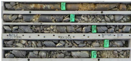
Composite 7 – 37.8 to 43.5m Coarse Disseminated Iron
