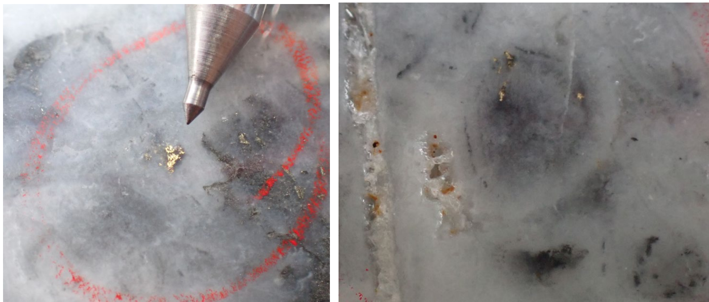
Photo 1: Visible gold mineralisation intersected in ARDH027 (interval 217m to 218m) which assayed 1m @ 79.1g/t Au. Fields of view for each photo approximately 2cm. Note the spherical quartz texture in the right-hand photo, considered to be a common texture associated with bonanza gold zones in many large epithermal and epizonal gold deposits.
