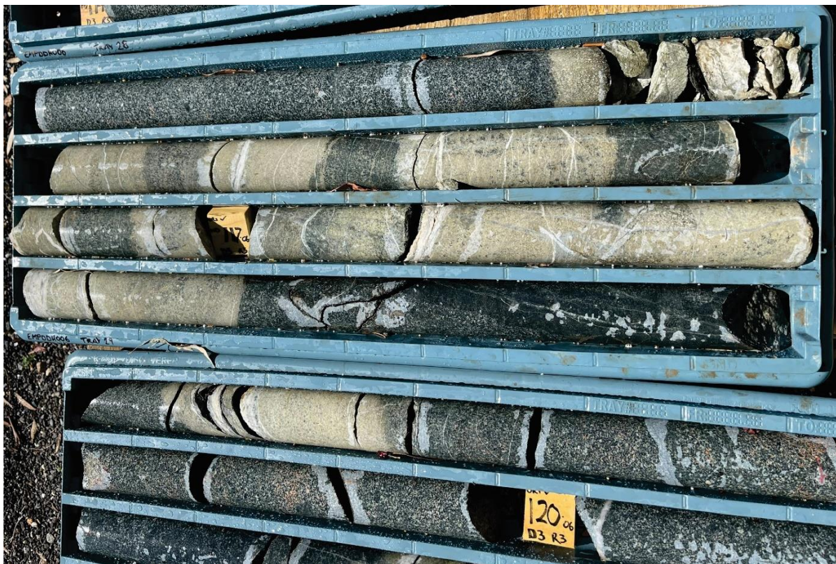
Figure 3 – Core from EMDDH006 between ~114.7 – 120.3m showing phyllic alteration. Fine, disseminated chalcopyrite and pyrite are common through the core, with molybdenite present in quartz veins.
