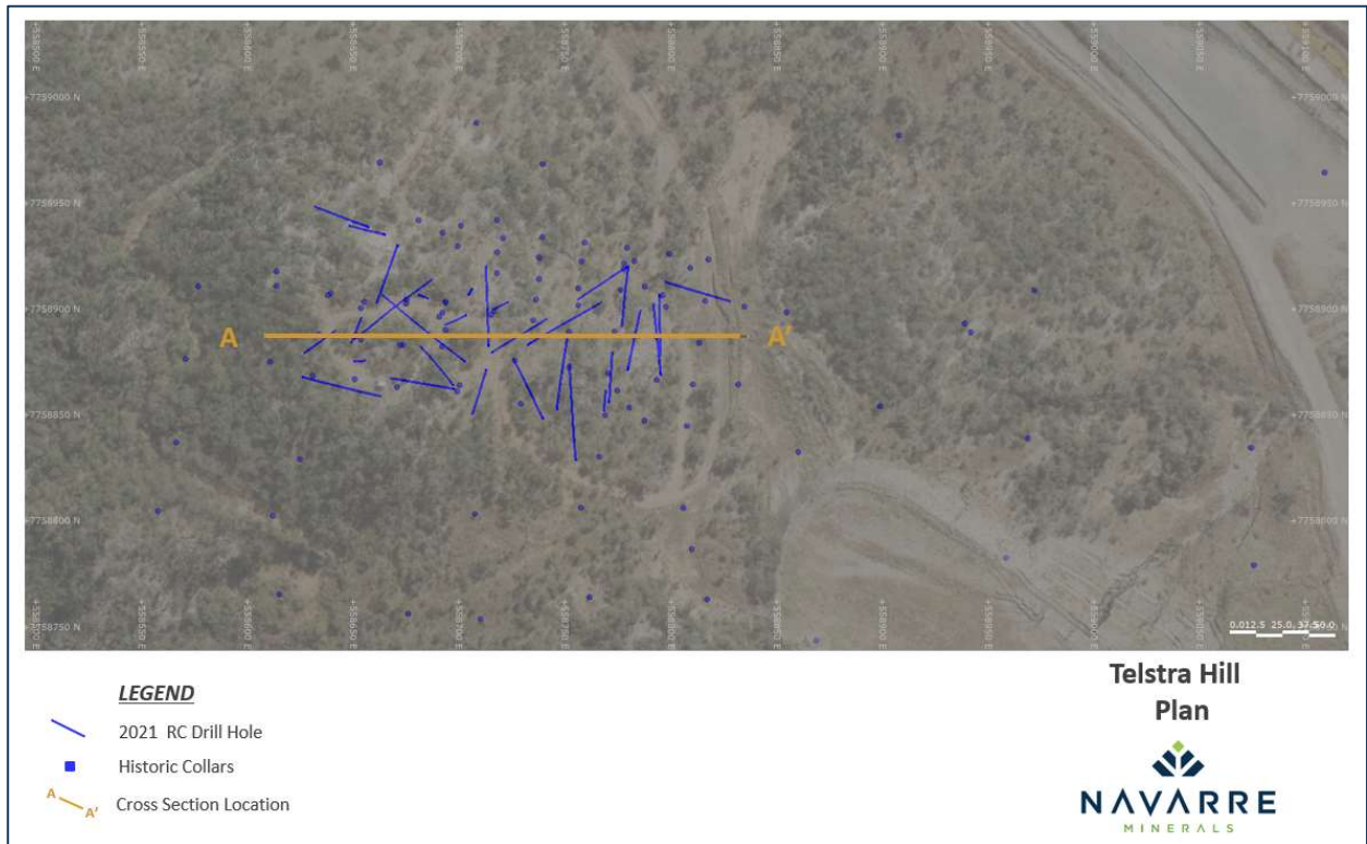
Figure 3: Plan of Telstra Hill showing the distribution of 2021 drill holes relative to historical drill collars. The location of the Figure 4 cross-section is shown in orange.
