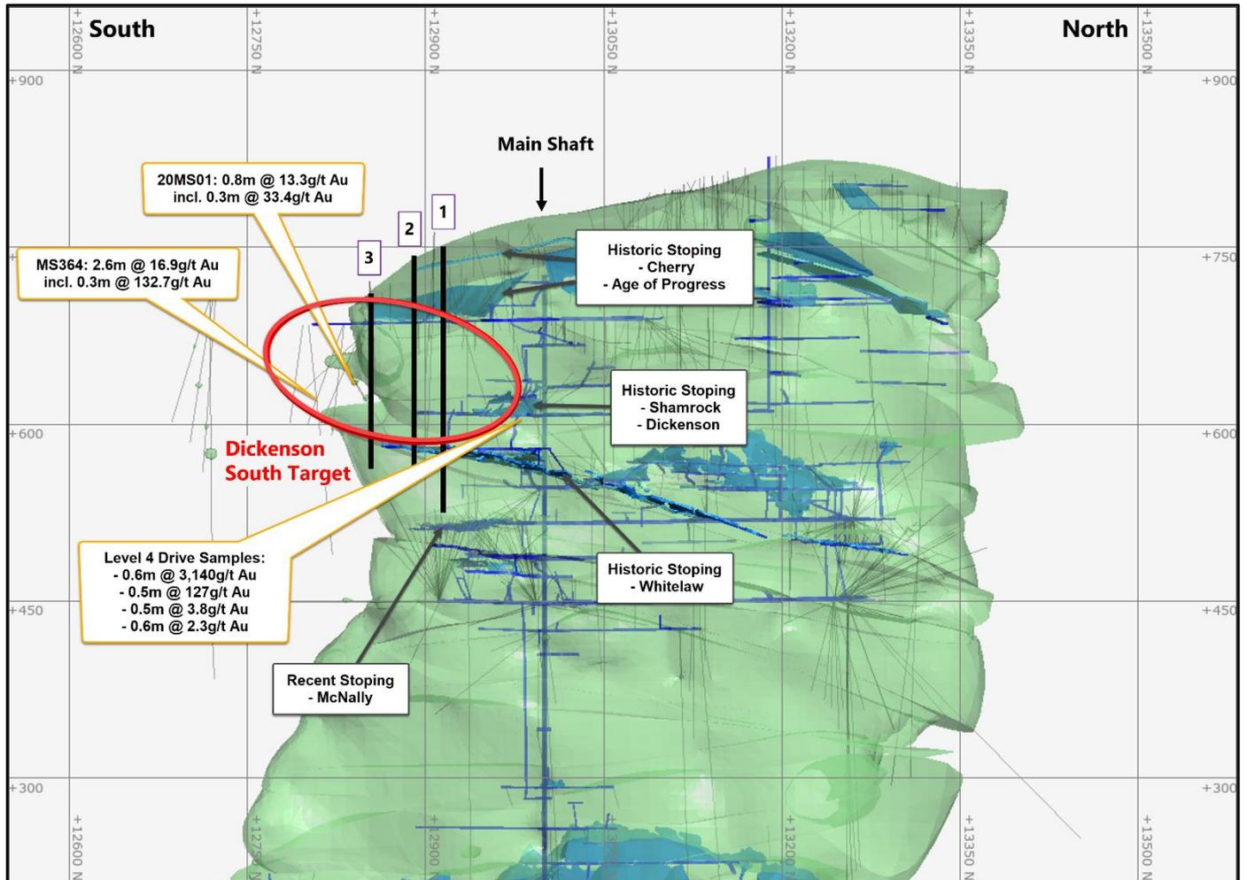
**Figure 2:** Long section view looking west highlighting the Dickenson South target area and the location of three rings of drillholes including 22SDS001 to 22SDS011. The long section view shows the host dyke, historic stoping and mine development and all drill hole traces, with historic drill hole intersections (downhole widths) and underground sampling that highlight the Company's interest in the Dickenson South target area.
