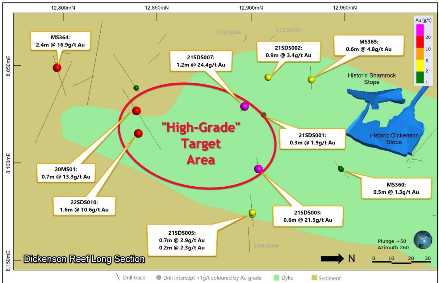
**Figure 1:** Long section view through the Dickenson reef showing current and historic true width drill intersection pierce points, the limited historic stoping and the potential "high-grade" target area at the southern end of the dyke.
