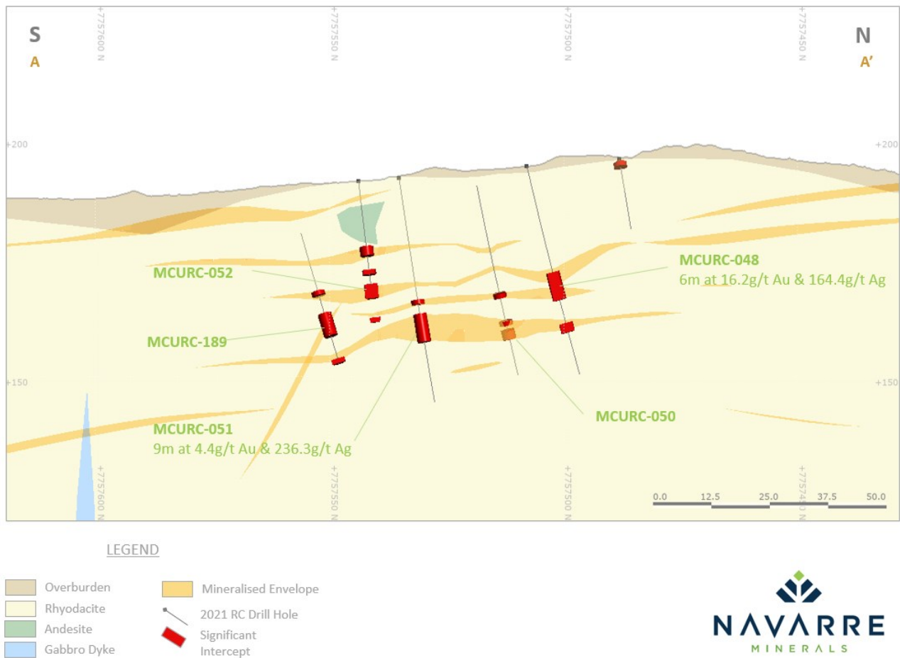
Figure 1: Schematic cross-section across Mount Carlton United
