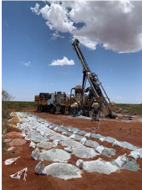
Photo 3: Strike Drilling T450 Aircore/Reverse Circulation Rig
