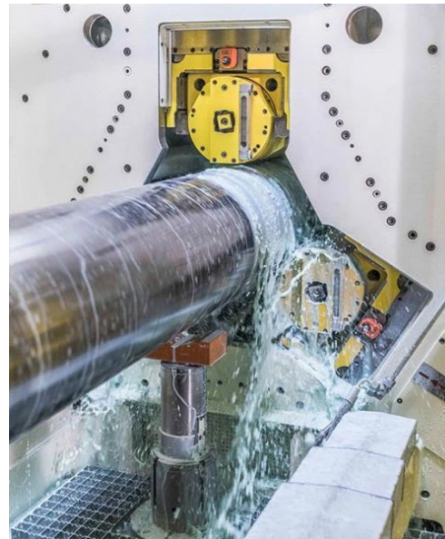
Repkon's flowforming technology
