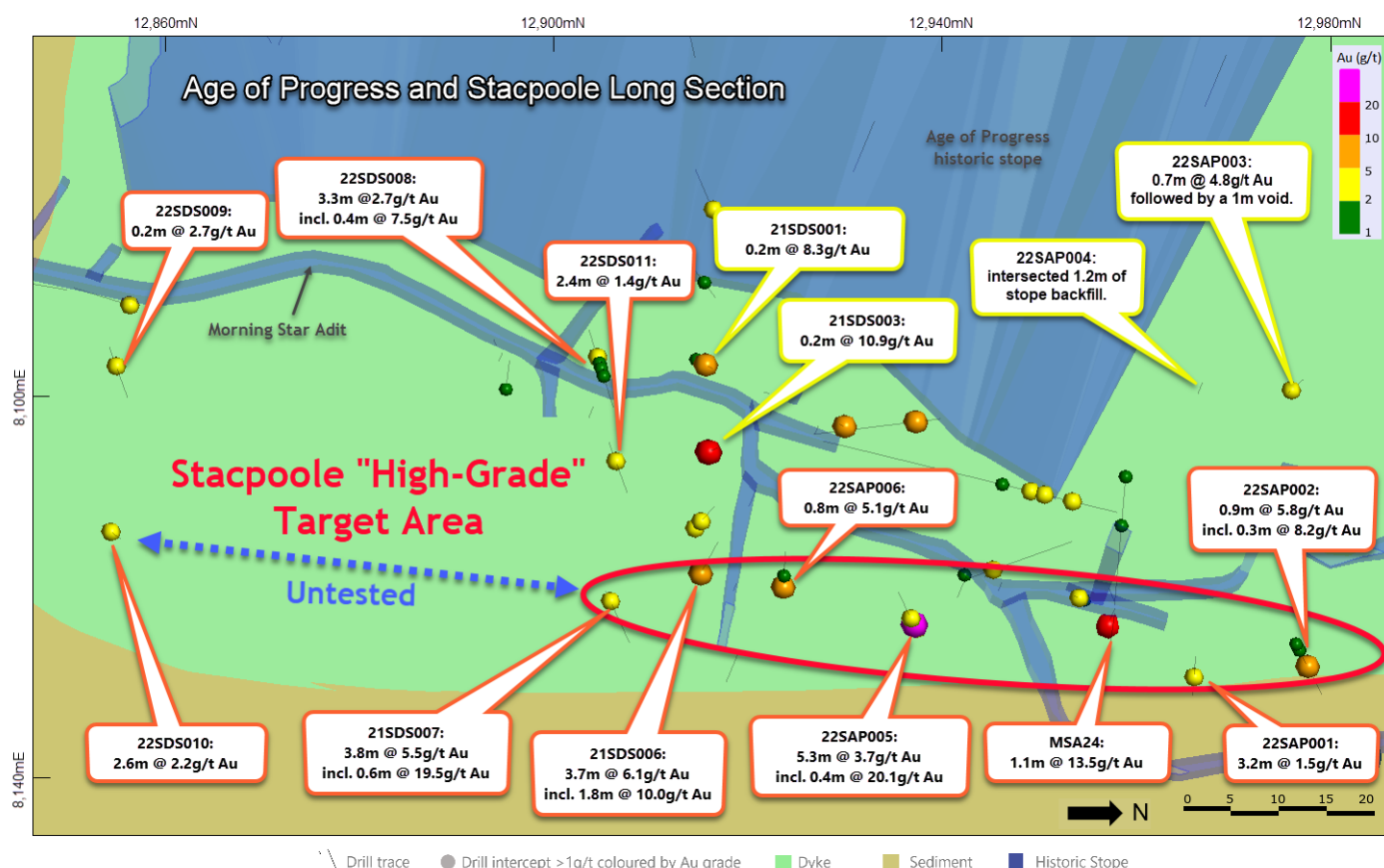
Figure 1: Long section view through the Stacpoole Reef showing current and historic true width drill intersection pierce points, the limited historic stoping on the Age of Progress Reef and the potential "high-grade" target area along the eastern edge of the dyke where the Stacpoole and Age of Progress Reef come together (refer Figure 3). Stacpoole Reef intersections outlined in orange and Age of Progress intersections outlined in yellow.
