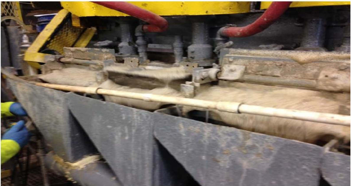
Figure 10 – Carbonate Rougher Flotation
