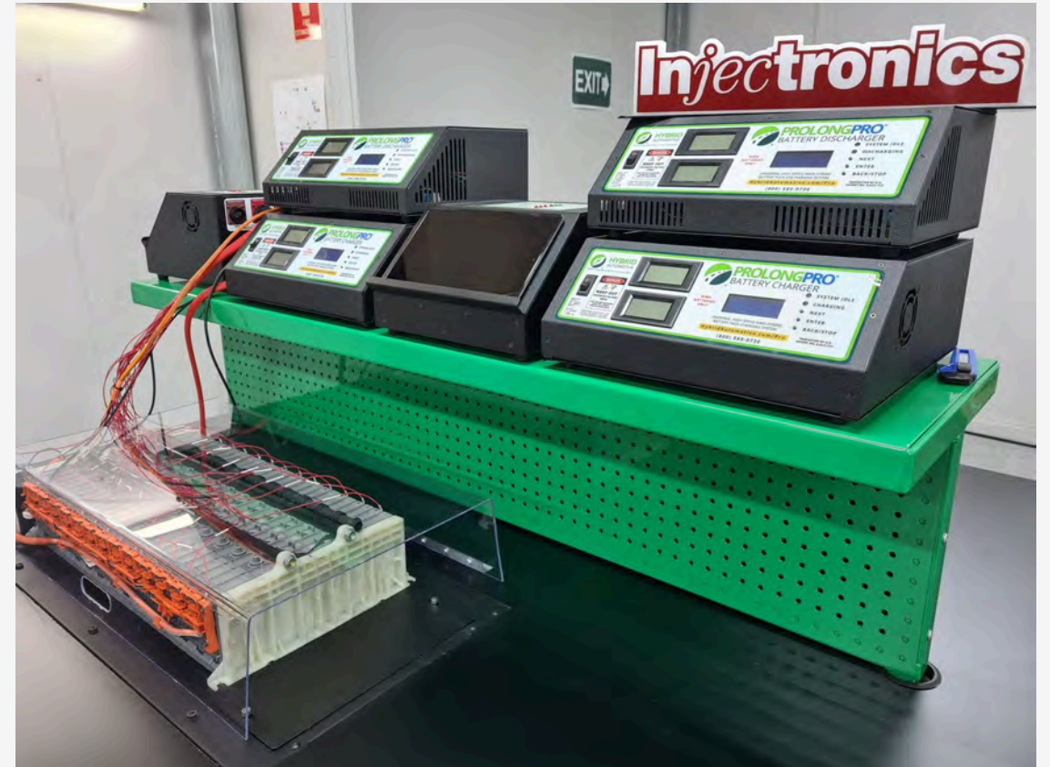
Hybrid electric vehicle battery diagnostics and rebalancing station
