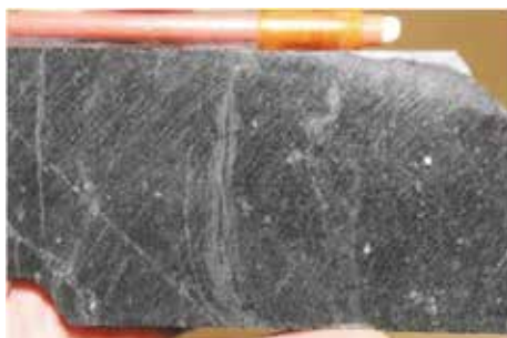
Plate 21. Biotite-magnetite altered volcaniclastic cut by magnetite-bearing M vein, 235.1m YS001RCD.
