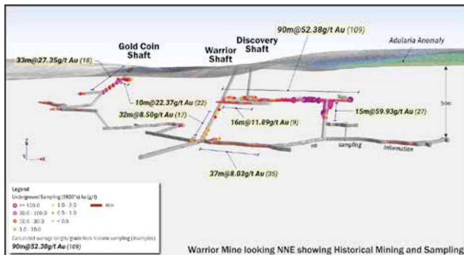
Figure 38. Plan view of SNG's 3D model of the Warrior Mine workings and sampling with Adularia intensity map in background. Note the bonanza grades returned from historic sampling underground of remnant vein material. Some of the better vein composites labelled. Composite grade is increasing to the SE towards the surficial Adularia anomaly (potassic core of the system). Interestingly the workings appear to have skirted around the edge and stopped short of the Adularia anomaly (UTM Zone 11 – NAD27 coordinates).
