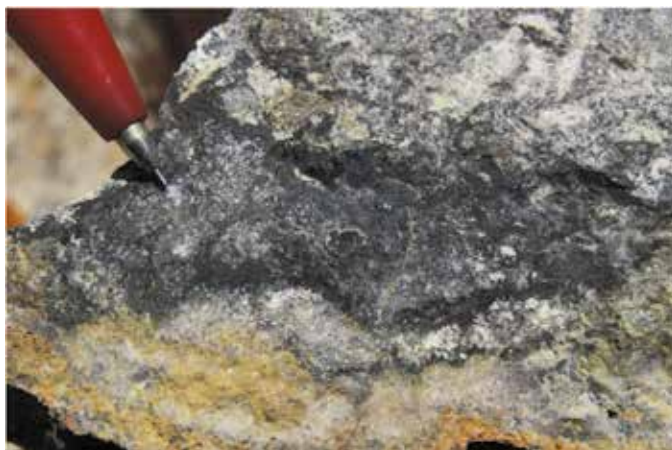
Plate 32. Bonanza grade vein from Morning Star Mines with silver sulphosalts within an opaline quartz vein which reported +1% silver, 5.78g/t gold, 14.85% lead
