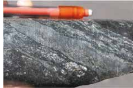
Plate 30. Laminated quartz-magnetite-actinolite-pyrite ± chalcopyrite bearing M-style vein in biotite-magnetite altered volcaniclastic breccia, 370.5m YS002RCD.
