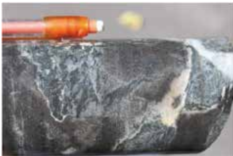
Plate 25. Quartz-actinolite-pyrite \pm chalcopyrite vein with K-feldspar selvage in biotite-magnetite altered volcaniclastic breccia, 328.8m YS002RCD.
