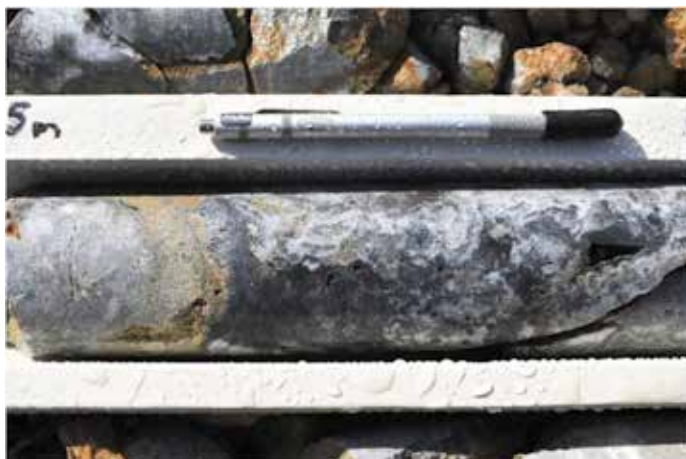
Plate 31. SNG Discovery Hole BDH006 intersected banded quartz, yellow-red sphalerite, galena, and Mn oxide after rhodochrosite. This photo from 259.5m which reported 1m at 243g/t silver, 0.54g/t gold, 7.03% lead, 14.65% zinc.
