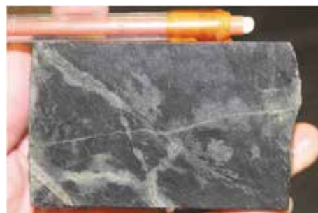
Plate 22. Biotite-magnetite altered volcaniclastic cut by quartz-epidote vein, 269.4m YS001RCD.
