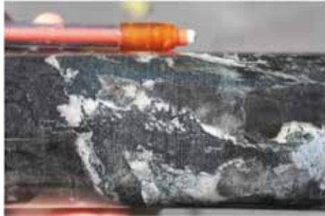
Plate 29. Fibrous actinolite-quartz-albite-chalcopyrite “squirts” in biotite altered volcaniclastic breccia, 321.1m YS002RCD
