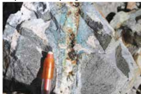
Plate 20. Quartz-malachite bearing B-style veins in siltstone, Falcon Target
