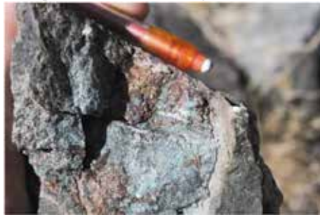
Plate 12. Quartz-chalcopyrite-bornite-actinolite bearing vein in andesite, Marietta Mine.
