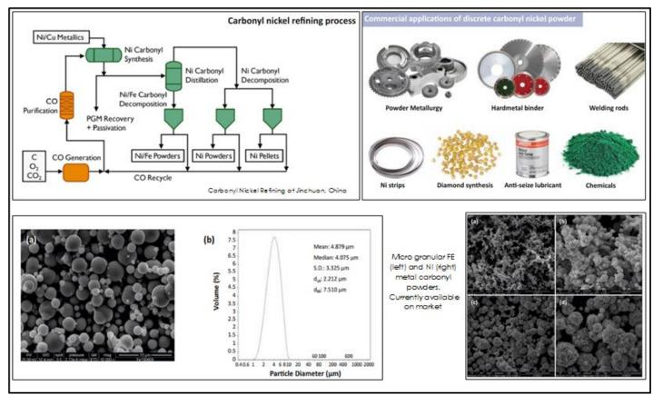
Figure 1: Carbonyl nickel refining process.
