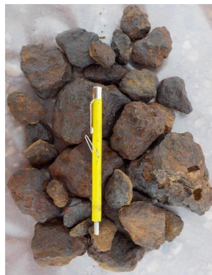
Figure 8 Location of rock chip sample TA272, assay number V2121, average iron grade 60.31%.
