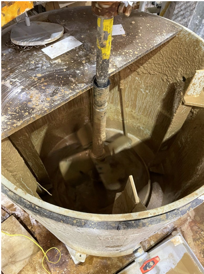
Figure 3 (Above) – Uranium rich solution from bulk leaching trials at ANSTO Minerals.
