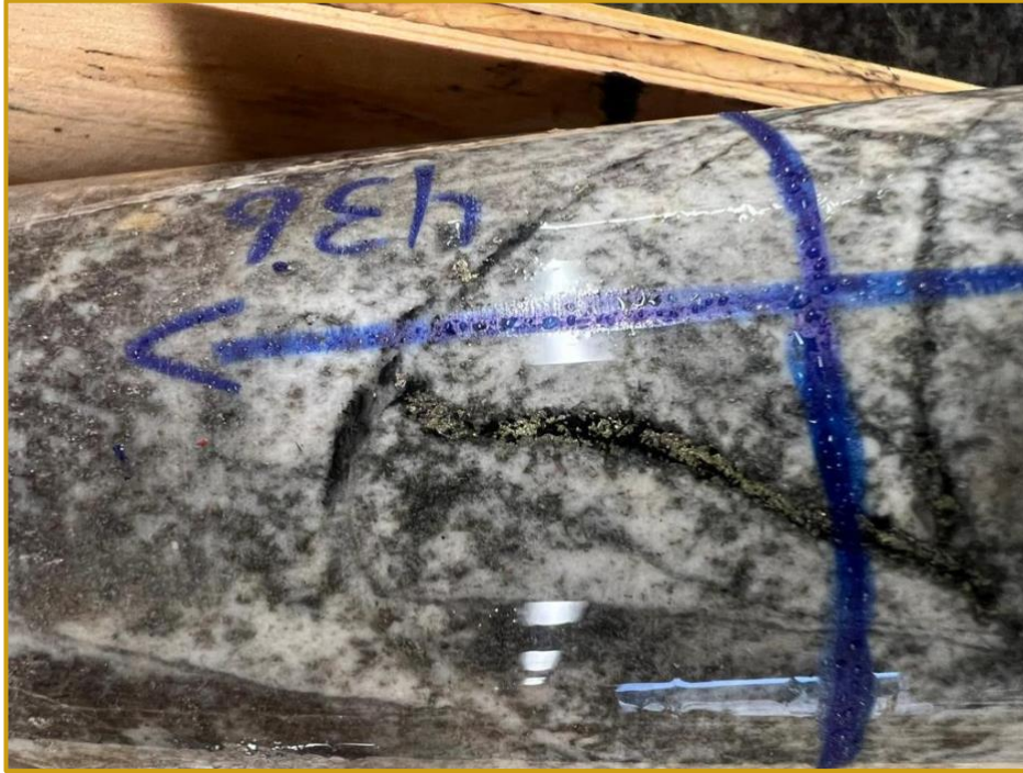
Figure 8. RPM-007 132.9m Strongly mineralized bleached hornfels with abundant sulfide veining and disseminated throughout rock.
