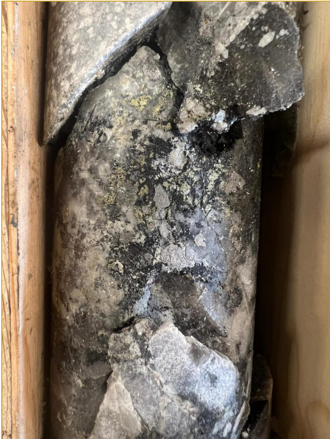
Figure 11. RPM-008 106.7m – Strongly mineralized chunky quartz-sulfide veins within grano-diorite intrusive units. Contains arsenopyrite and tourmaline typical positive indicators for high grade gold.
