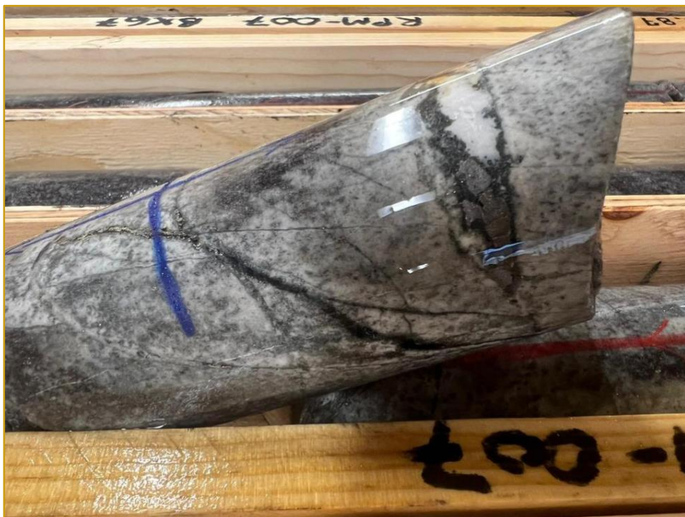
Figure 7. RPM-007 130.8m Strongly mineralized bleached hornfels with chunky arsenopyrite
