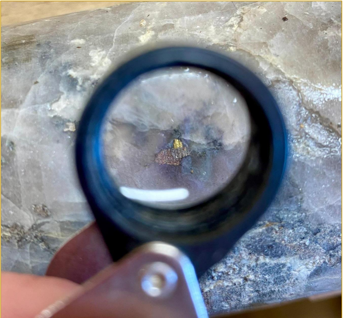
Figure 12. RPM-008 115.8m – Visible Gold in a quartz-sulfide vein within intrusive rocks.
