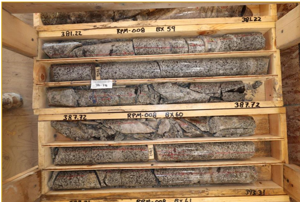
Figure 9. RPM-008 116.2-119.9m Strongly mineralized thick quartz-sulfide veins within grano-diorite intrusive unit. Previous drillhole assay results have shown this material contains some of the highest grade zones at RPM North. (Note: depth written on boxes in feet)
