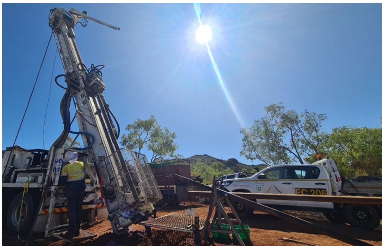
Figure 1: MI22DD01 diamond drilling, Millennium Southern Area
