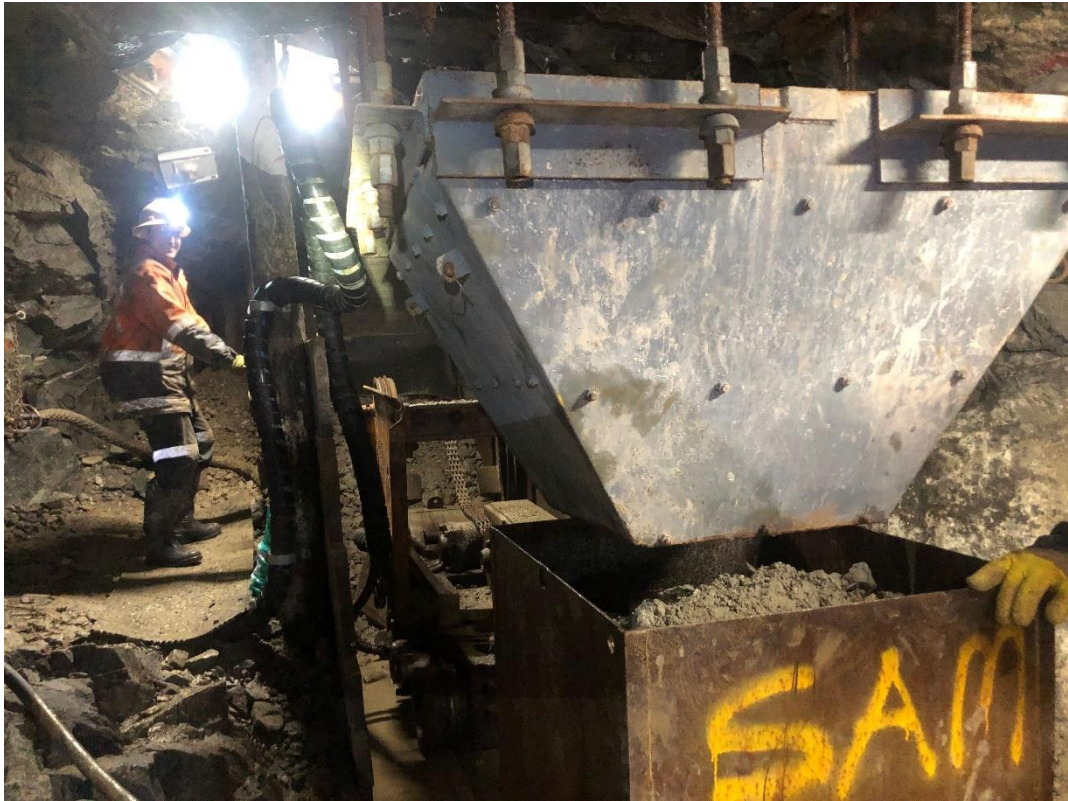
Figure 9: Compressed air rocker shovel (loader) on the main haulage 9 Level loading broken material into an ore “truck”
