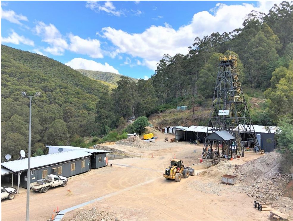
Figure 11: Morning Star mine site with headframe and winder on the right and offices to the left
