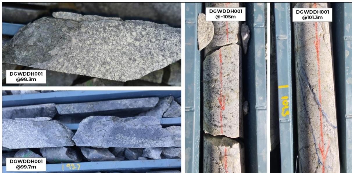
Figure 2: Porphyry intersected in DGWDDH001 from 88.9m to 110m displaying disseminated, fly-speck and veined chalcocite mineralisation.
