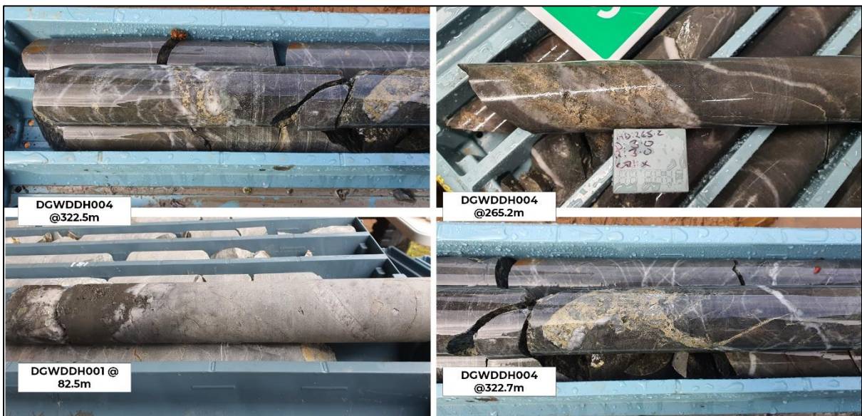
Figure 4: Variable sulphide mineralogy including chalcocite, chalcopyrite and pyrite sulphides observed in drillholes DGWDDH001 – DGWDDH004 holes.
