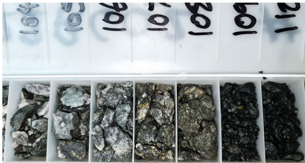
Figure 6: Copper-rich interval in RC drill chips showing (MI22RC02) moderate to abundant chalcopyrite in highly altered silica-biotite metasediment (left) adjacent carbonaceous siltstone (right)
