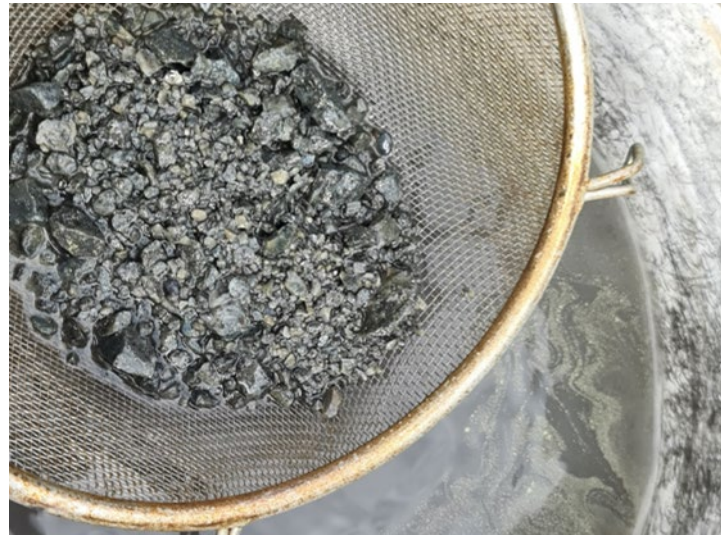
Figure 5: Copper-rich interval in RC drill chips showing abundant chalcopyrite in siliceous metasediment
