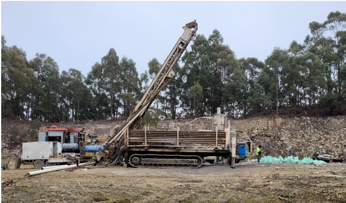
Figure 4. Scout RC drilling of hole KERCO01 at Kensington located within an abandoned quarry.
