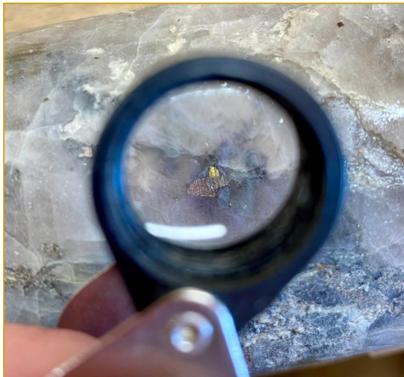
Figure 4. RPM-008 115.8m – Visible Gold in a quartz-sulfide vein within intrusive rocks.
