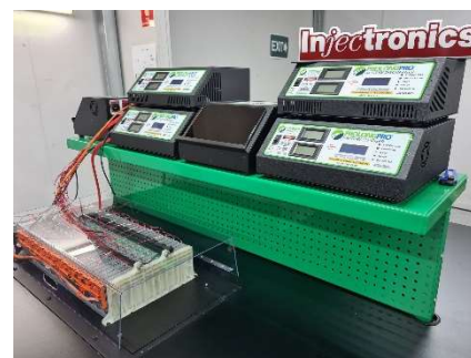
Hybrid EV battery testing station
