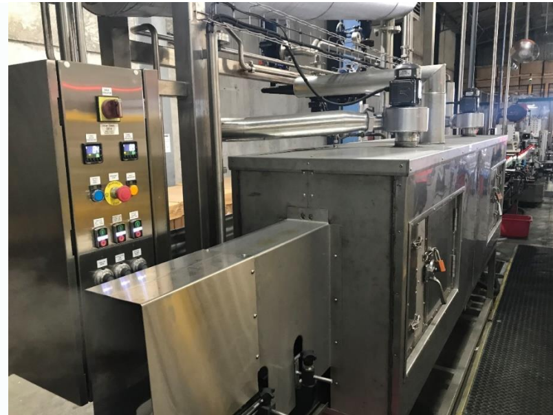
NEW sleeving tunnel in bleach plant
