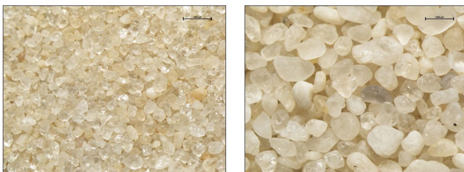
Figure 1 – Photomicrograph images of the Upper White sub domain, Left, image is -0.60mm to +0.15mm, right image is -1.0mm to +0.60mm (Bar line in the upper right is 1mm)
