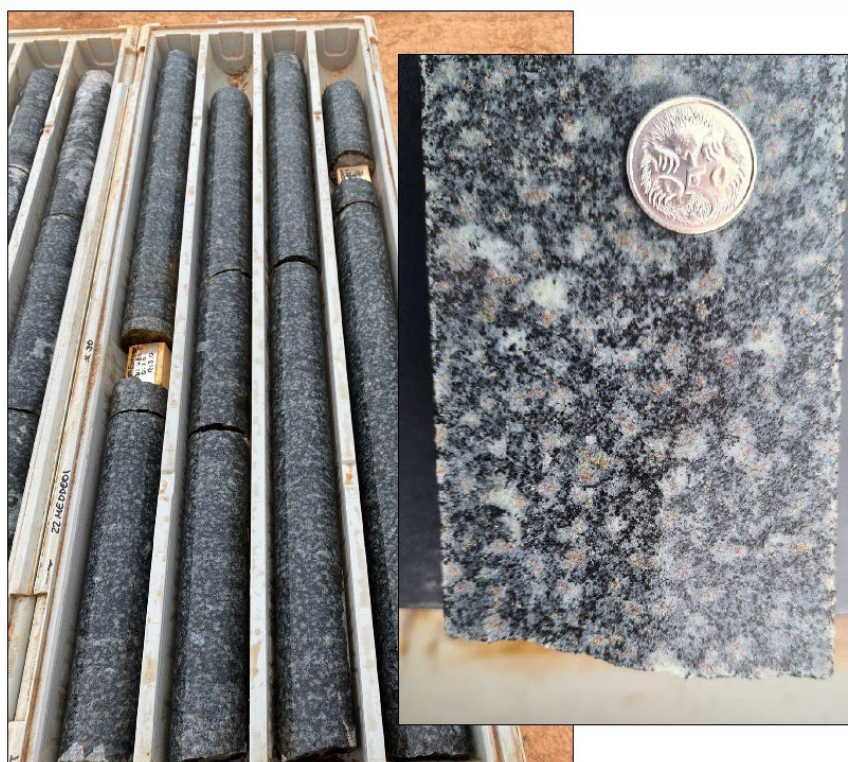
Figure 6. 22MEDD001, 595-605m, oxidised weathered low angled fault zone.
