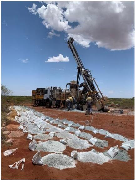
Photo 2: Strike Drilling T450 Aircore/Reverse Circulation Rig
