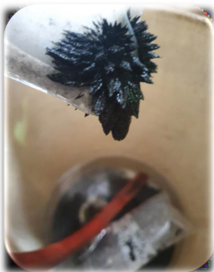
Figure 9: Magnetic Concentrate - Magnetic particles attracted to a hand magnet from the upper saprolite.
