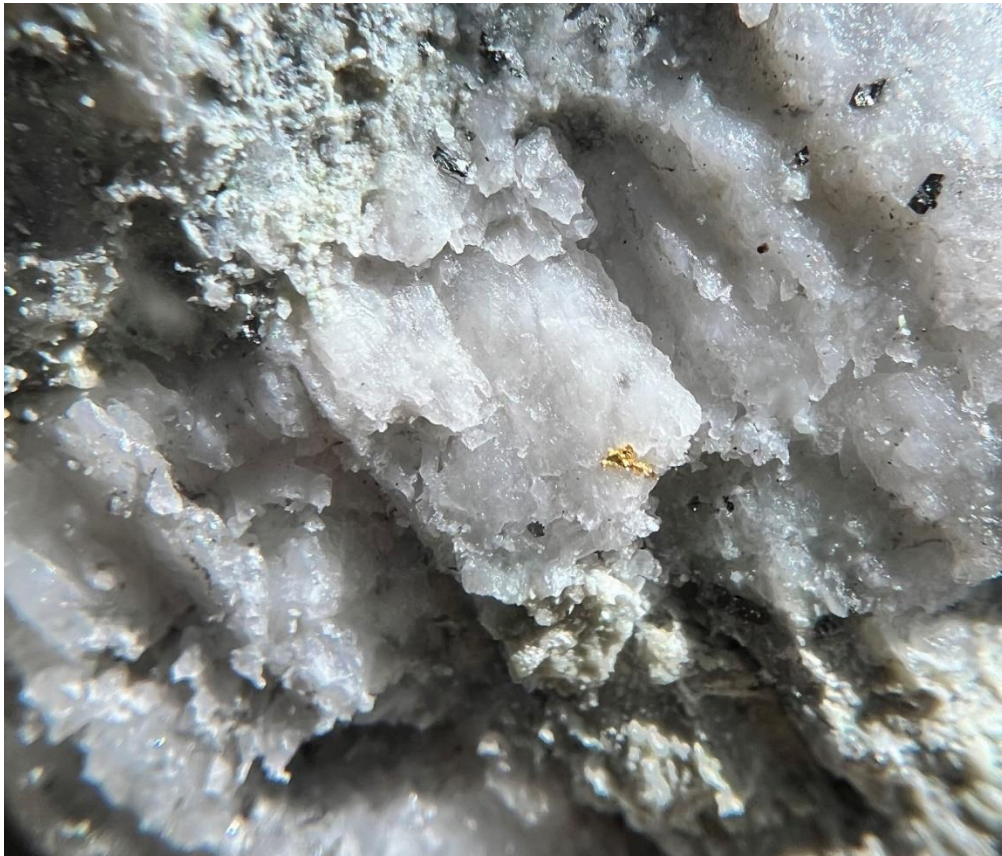
Photo 2: SDDSC049 211.9m, field of view 20mm, with visible gold within quartz.
