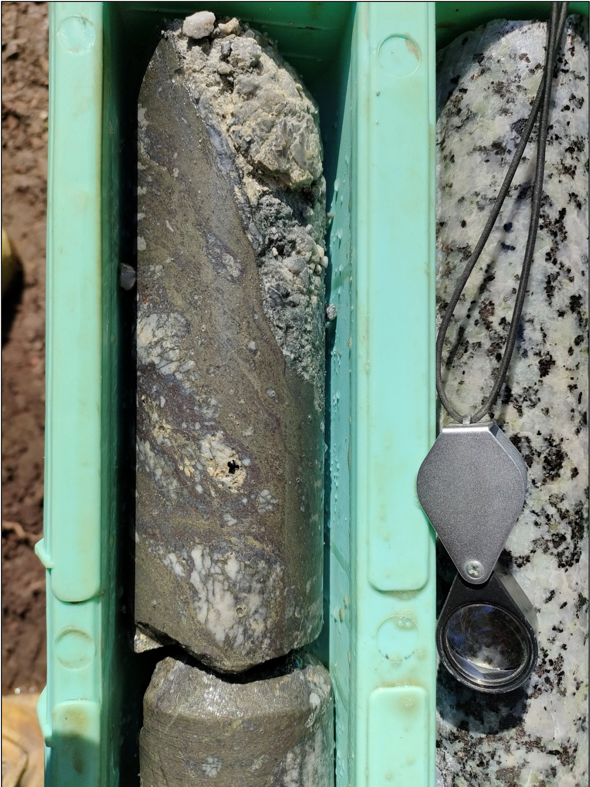
Plate 1: Massive sulphide-quartz vein mineralisation which graded 0.5m @ 143.0g/t Au from 57.5m in TFDD003.
