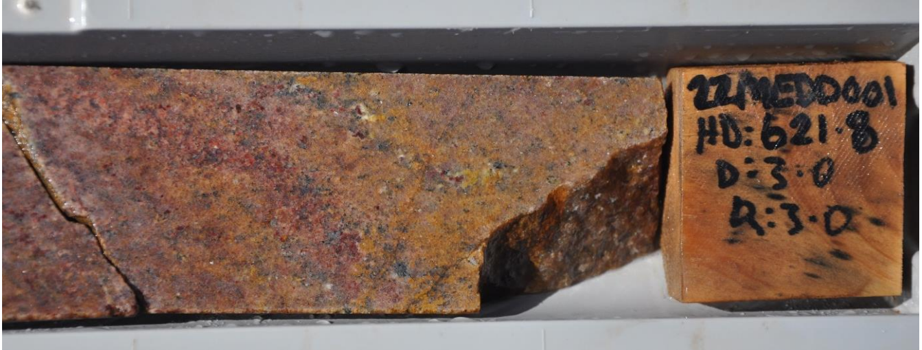
Figure 4: 22MEDD001 hematite, albite, sericite, chlorite, epidote, and pyrite alteration in syenogranite at 621.6m
