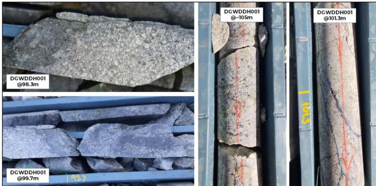
Figure 1: Porphyry intersected in DGWDDH001 from 88.9m to 110m displaying disseminated, fly-speck and veined chalcocite mineralisation.
