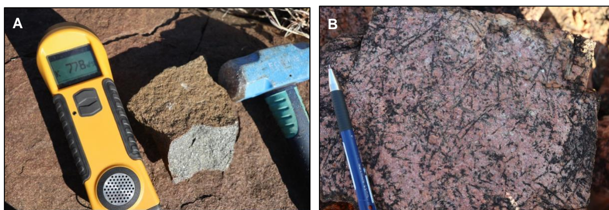
Figure 8. A) Disseminated magnetite gabbro sample and B) felsic differentiated sample that are prospective target horizons for V-Ti and Ni-Cu-PGE mineralisation.
