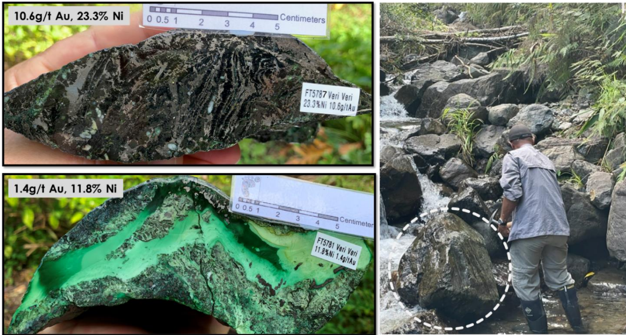
Photo 2: Veri Veri creek float samples include massive nickel sulphide minerals (heazlewoodite, millerite, pentlandite) and nickel-bearing silicates including serpentinite and garnierite. Photo Right: boulder with nickel sulphides in creek. Samples taken by Footprint, see Table 4 and JORC tables in this announcement.
