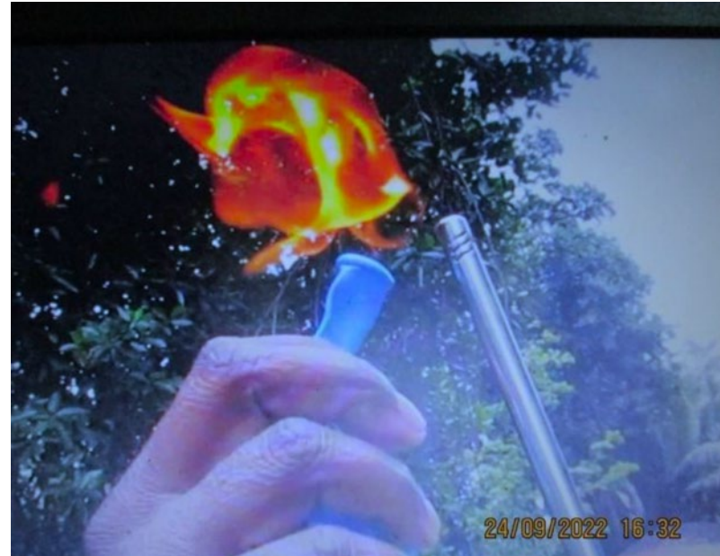
Field-test of gas bubbling from reservoir
