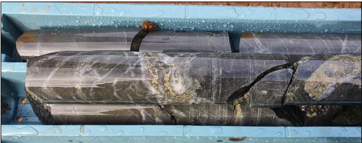
Figure 2: A chlorite-epidote altered chalcopryrite sulphide quartz vein overprinting potassic biotite-magnetite veins from 322m in Hole 4
