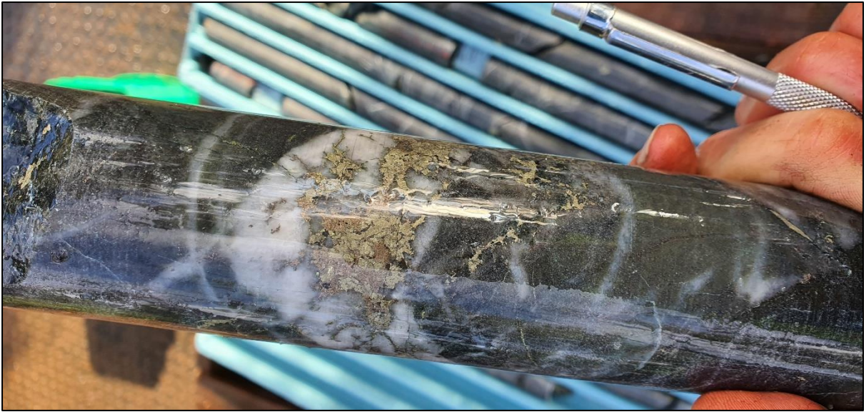
Figure 1: Chalcopryrite + Pyrite + Quartz veins from Hole 4 @ 322.5m
