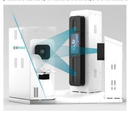
The XV Scanner is a unique piece of hardware specifically designed to utilise 4DMedical's proprietary XV Technology® on a pay-per-scan basis. It overcomes the limitations of existing diagnostics and imaging tools by providing low dose, contrast-free, rapid lung analysis. The device delivers detailed quantitative data on respiratory function via an automated scanning process, providing unprecedented insight to clinicians, researchers and patients.
